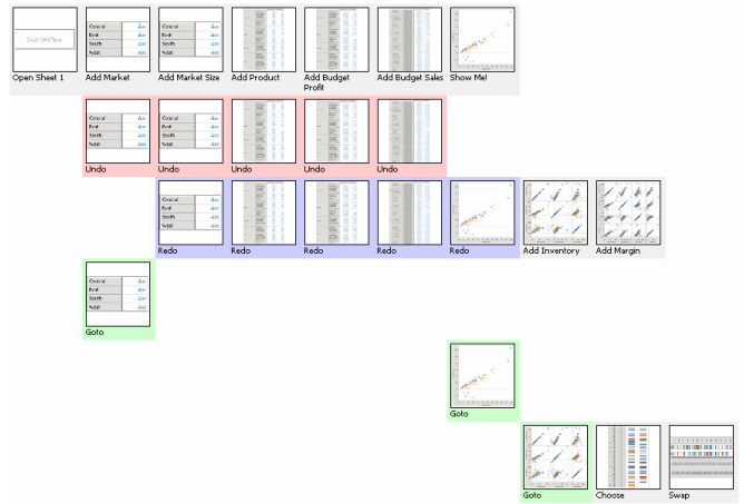
Fig. 9. Tableau Behavior Graphs depict user behavior in an analysis session. Actions except undo and goto are placed sequentially in left-to-right order. Undo actions (red) move right-to-left on a new row. Goto actions (green) indicate navigation actions made in the history viewer.
