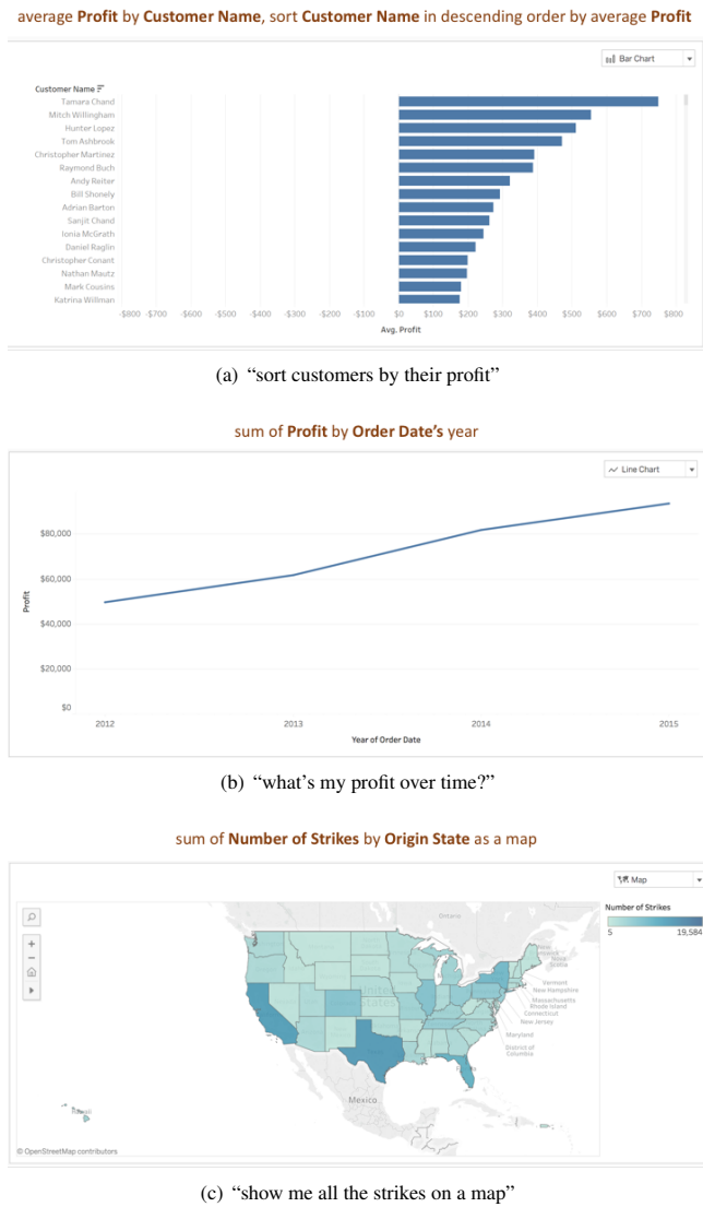
Figure 1: System inferences made for underspecified utterances during visual analysis. (a): Infers a descending sort order to sort Customer Names by Profit . (b): A user expresses an intent of ‘time’ that is resolved to a time attribute Order Date aggregated at its year level. (c): Infers a geographical attribute, State , in order to display the number of bird strikes in a map employing user popularity data and heuristics for analytical usefulness. Note: The canonical form is displayed on top of each figure for legibility while the input utterance is shown in the caption.
