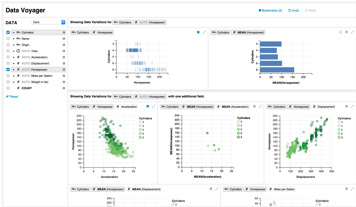
Fig. 1. Voyager: a recommendation-powered visualization browser. The schema panel (left) lists data variables selectable by users. The main gallery (right) presents suggested visualizations of different variable subsets and transformations.
